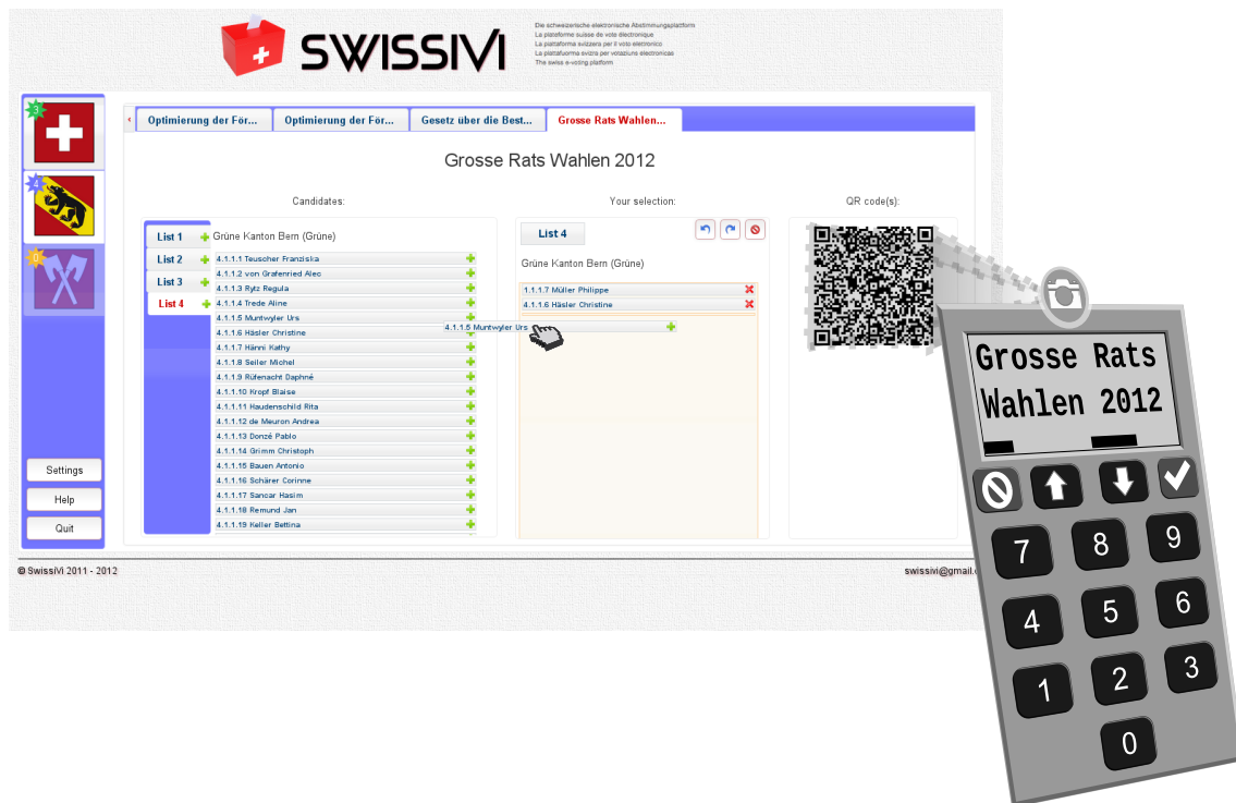
Figure 9.3.: The voting platform presents a highly interactive form of a complex election scenario. The matrix code keeps changing when a new selection is made. This superpositions the possibilities over time. The trusted voting device is used to capture the desired options. The image of the voting platform represents the look of the implementation in [88]
