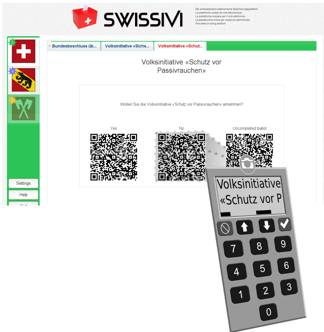
Figure 9.2.: The voting platform showing an initiative where all possible options are in superposition. The trusted voting device is then used by the voter to select a specific option. The image of the voting platform represents the look of the implementation in [88]
