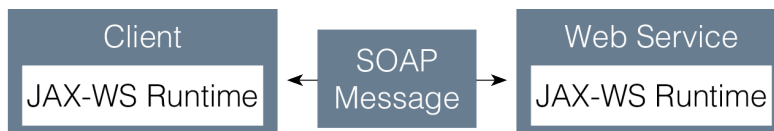
Figure 2: Communication between a JAX-WS Web Service and a Client [4]
